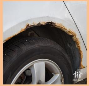
While road salt helps drivers get safely from one place to the next by keeping streets clear of ice and snow, repeated exposure can leave your vehicle vulnerable to rust. If not correctly taken care of, rust can cause significant damage to your vehicle and pose serious safety risks. Here are 5 things you can do to protect your vehicle from rust damage this winter. Read more at www.otip.com/article156.
